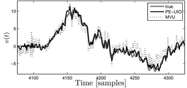
Fig. 1. Comparison of efficacy of PE-UIO and MVU ( $\sigma_u^2 = 1, \sigma_y^2 = 1$ )
